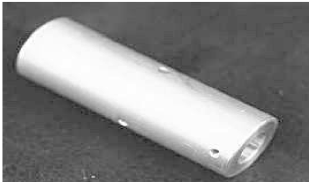
Fig. 2 Aluminum balance adapter used in the model.
